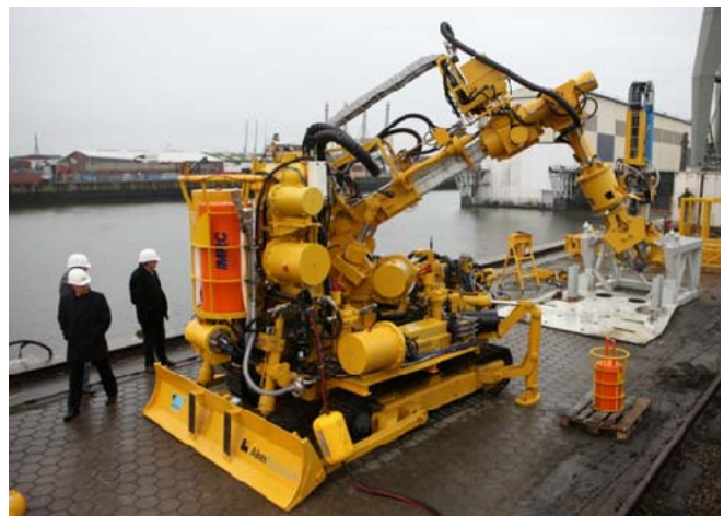
Figure 7: The IMPaC-dCAS subsea boxes with the Seafloor Working Unit from Aker-Wirth during trials
