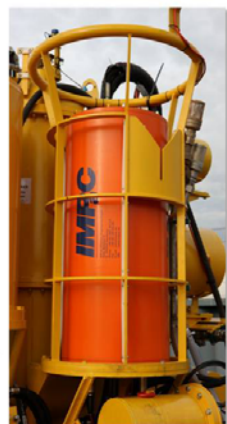
All electric Subsea Control Module for deep water application
