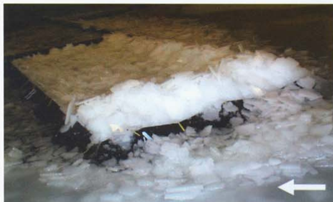
Fig. 7: Light-weight ice barrier with accumulated rubble ice and indicated ice drift direction
