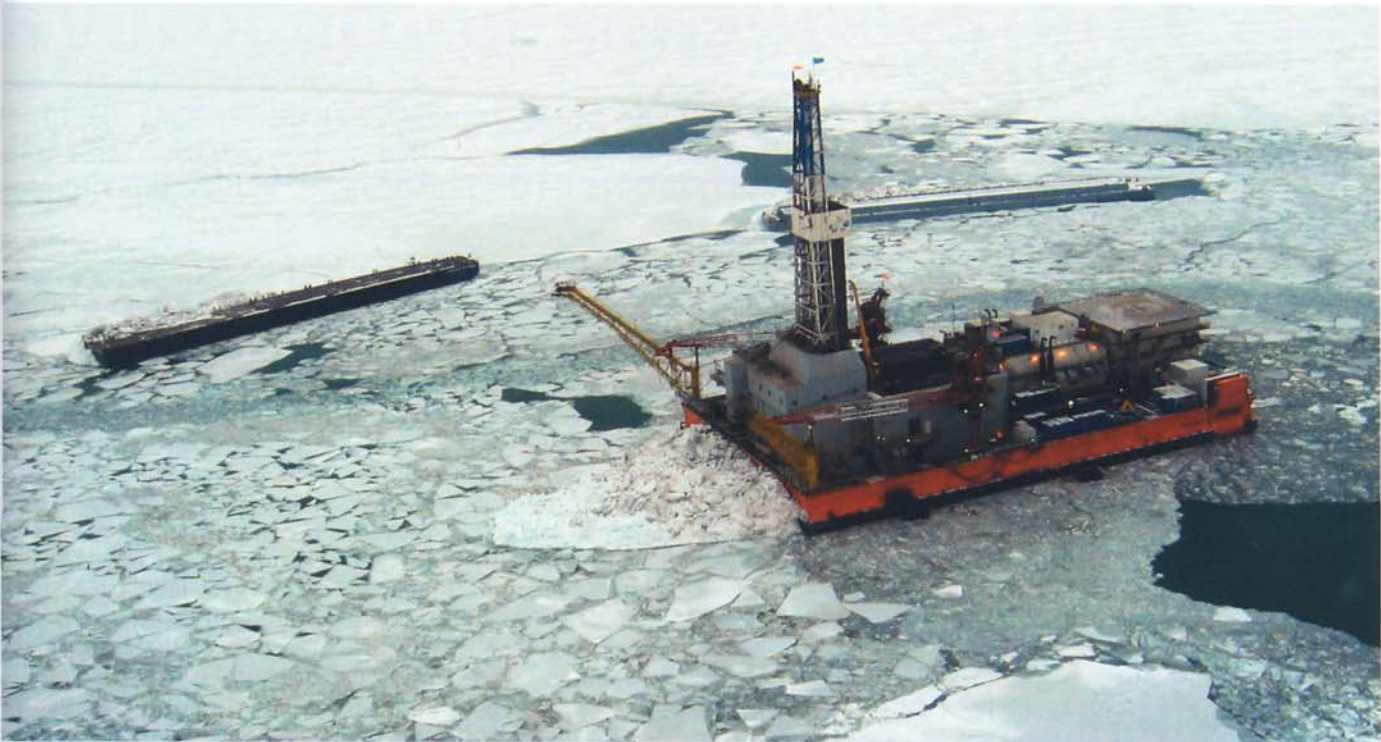
Fig. 3: Drilling unit with barge type ice barriers to protect against excessive ice loads
