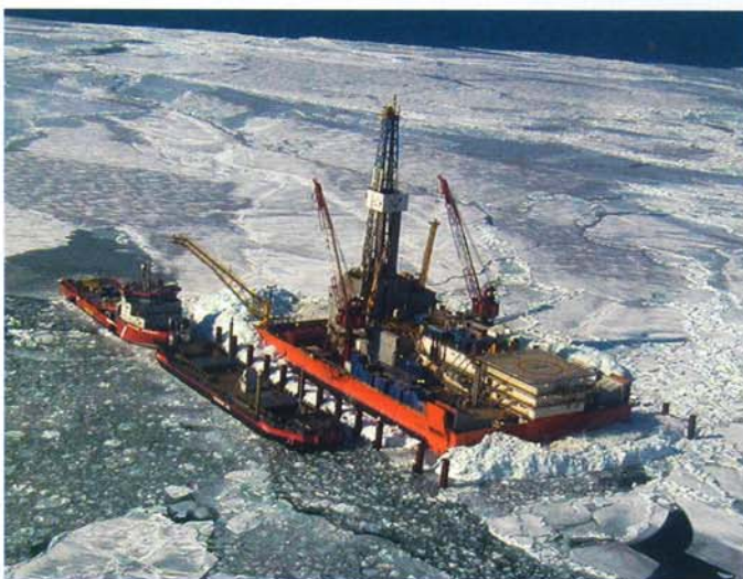
Fig. 1: Drilling unit with driven piles as ice protection structure
