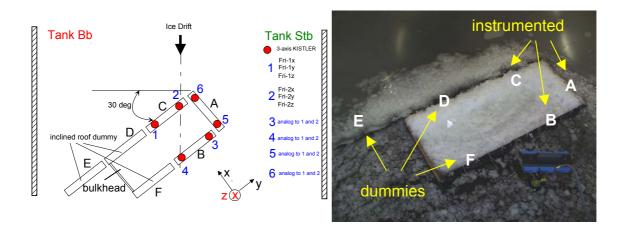
Fig. 7 Schematic of 'roof type" structure arrangement and instrumentation
