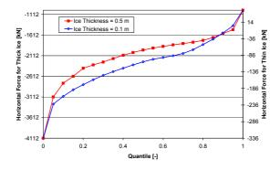
Fig. 11 Quantiles of horizontal forces for 0.1 m thick ice and for 0.5 m thick ice. Fig. 11 can be used to derive design loads for a specific safety level. The load distribution may be described statistically e.g. by a GUMBEL-distribution.
