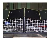
Fig. 5 'Roof type' structure with a net between vertical piles
