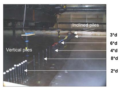
Fig. 1 Arrangement of vertical and inclined protection piles
